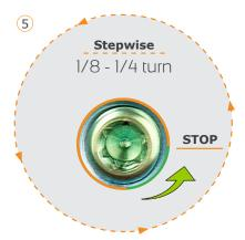
Hold till screw doesn't show counter torque, then next 1/8 - 1/4 turn
